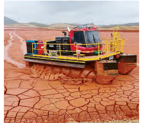
Amphibious Scrollers, which are designed and built in-house by the McCosker team. (Supplied)
