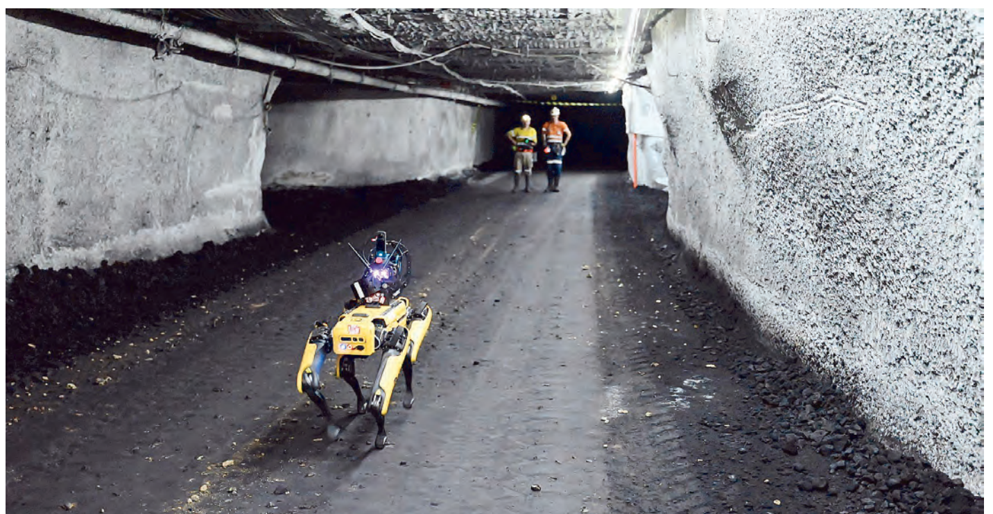
Boston Dynamics' robodog was trialled at Anglo's Moranbah North Mine as a potential tool to visually inspect Grosvenor Mine safely. (Supplied)
