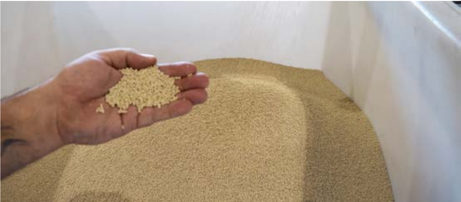
Waste plastic after it has gone through their on-site recycling plant, which is bagged and sent away to be re-used in the manufacture of other products
