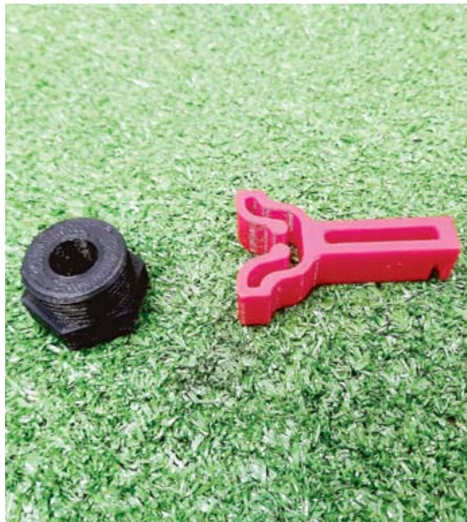
A pipe fitting (left) and an electric fence insulator (right) manufactured by the 3D printer at the Ken Coombe Tech Yards.
