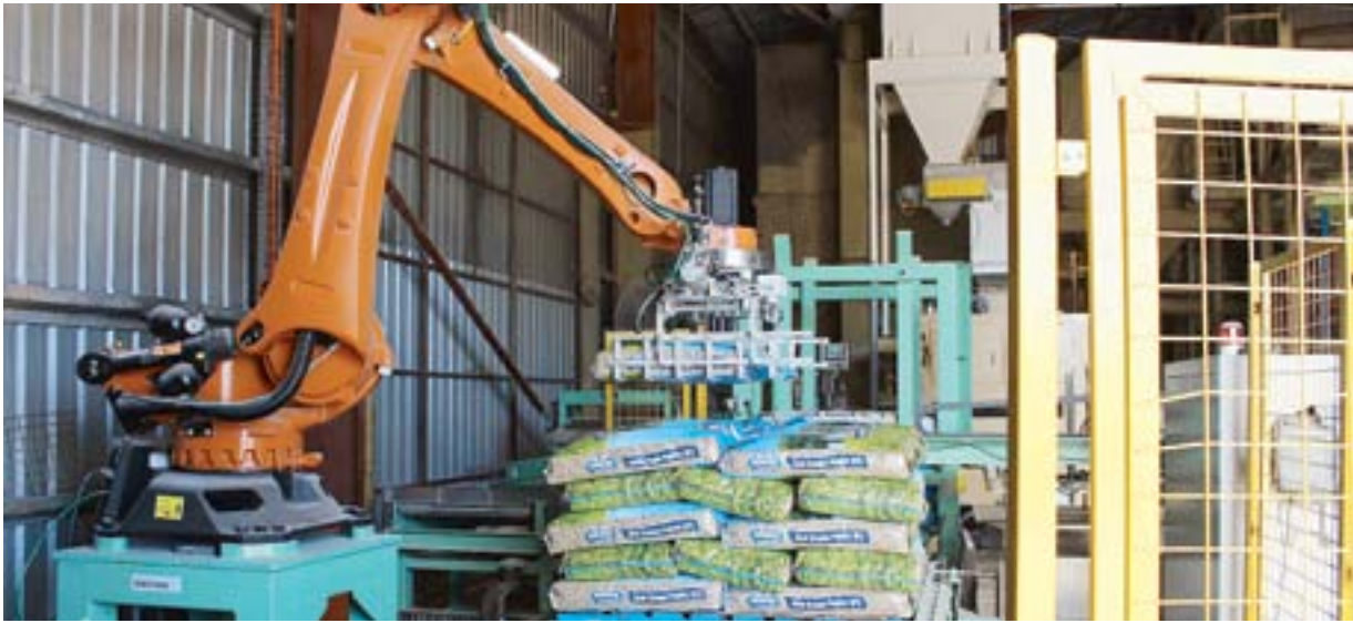
The mechanical arm at work at Blue Ribbon Stockfeeds.
