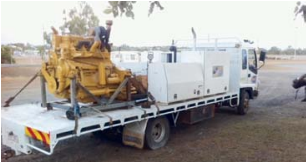
A re-built engine for a bulldozer. The engine is going back out to the machine to be installed.
