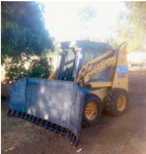
A stickrake built by RCM for a skid steer loader. Around 12 of these have been sold so far.
